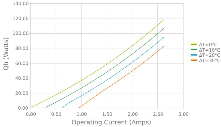
Total Heat Dissipated at Hot Side (Qh=Qc+Pin)
