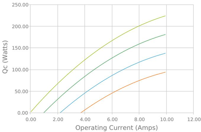
Heat Pumped at Cold Side ( $Q_c$ )
