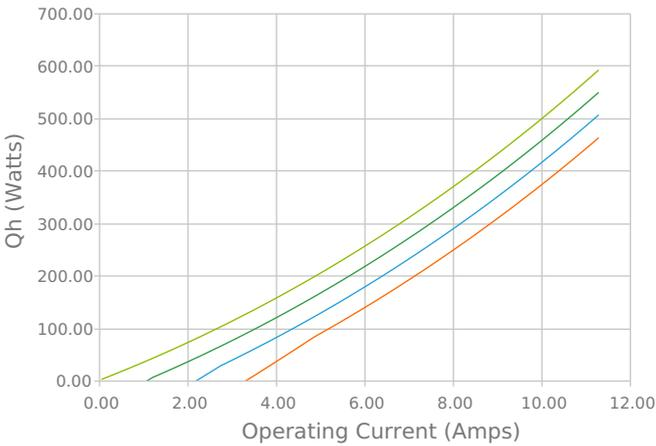
Total Heat Dissipated at Hot Side (Qh=Qc+Pin)
