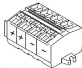
**Warning:** Do not reverse current or use PWM-regulation on fan supply.
