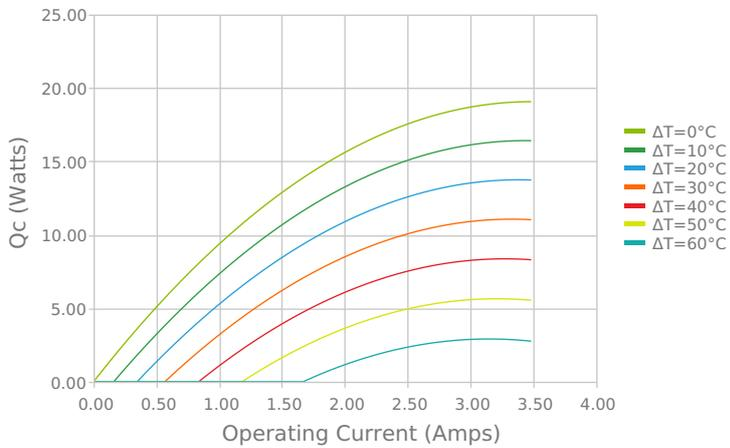
Heat Pumped at Cold Side
