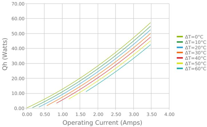
Total Heat Dissipated at Hot Side (Qh=Qc+Pin)
