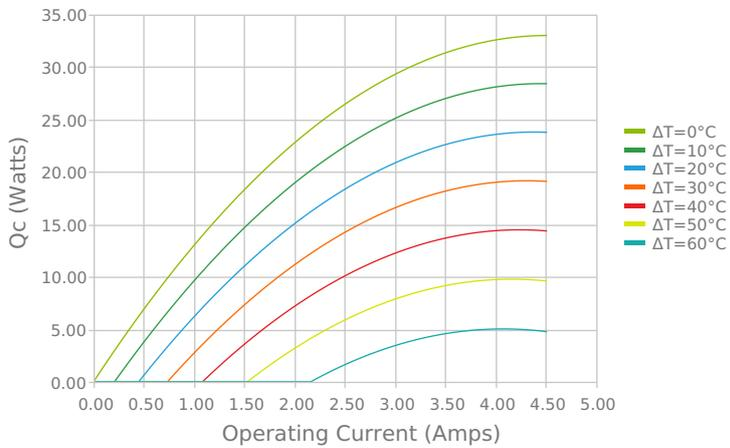
Heat Pumped at Cold Side
