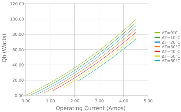
Total Heat Dissipated at Hot Side (Qh=Qc+Pin)
