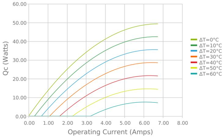
Heat Pumped at Cold Side
