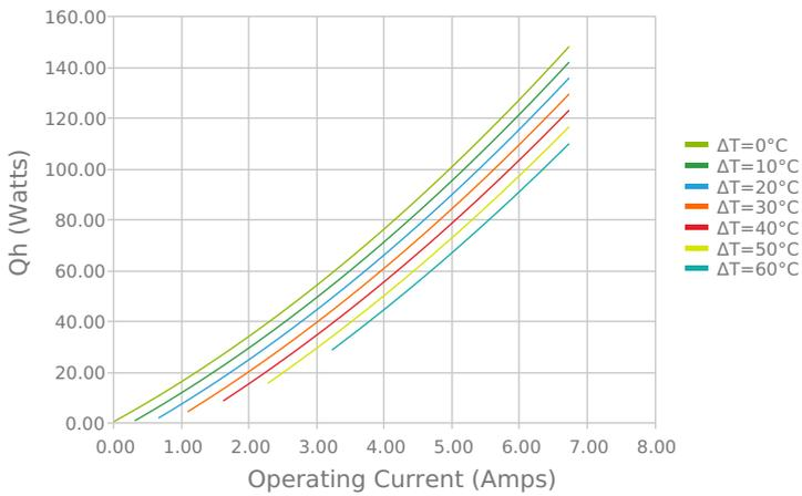
Total Heat Dissipated at Hot Side (Qh=Qc+Pin)
