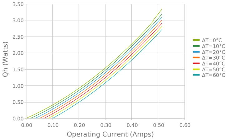
Total Heat Dissipated at Hot Side (Qh=Qc+Pin)
