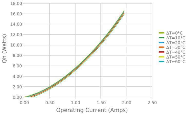
Total Heat Dissipated at Hot Side (Qh=Qc+Pin)
