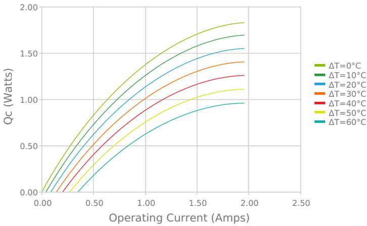
Heat Pumped at Cold Side
